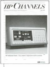
The HP 3082A Industrial Touch terminal is a small, rugged terminal that accommodates touchscreen, barcode, and keypad input for increased ease of use in today's CIM environment. See articles beginning on page 20.
